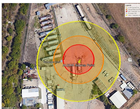
Figure 6. Thermal radiation zones generated by the butane jet fire.
