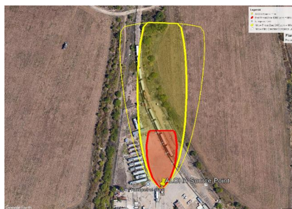
Figure 5. Dispersion of the propane cloud and the zones corresponding to the 60% and 10% LEL thresholds.
