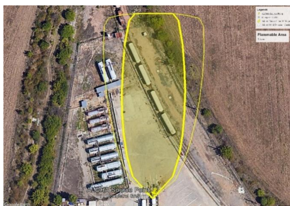
Figure 4. Dispersion of the butane cloud and the zone corresponding to the 10% LEL threshold.
