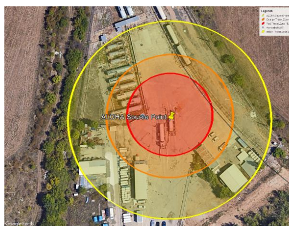
Figure 7. Thermal radiation zones generated by the propane jet fire.
