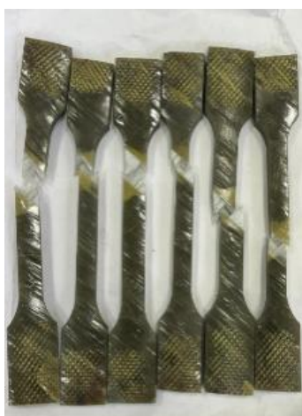
Figure 14. Test specimens after tensile testing
