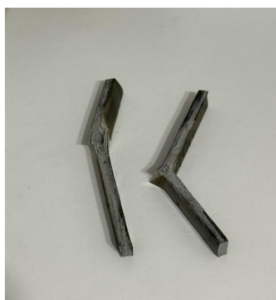
Figure 16. Test specimens after the bending test
