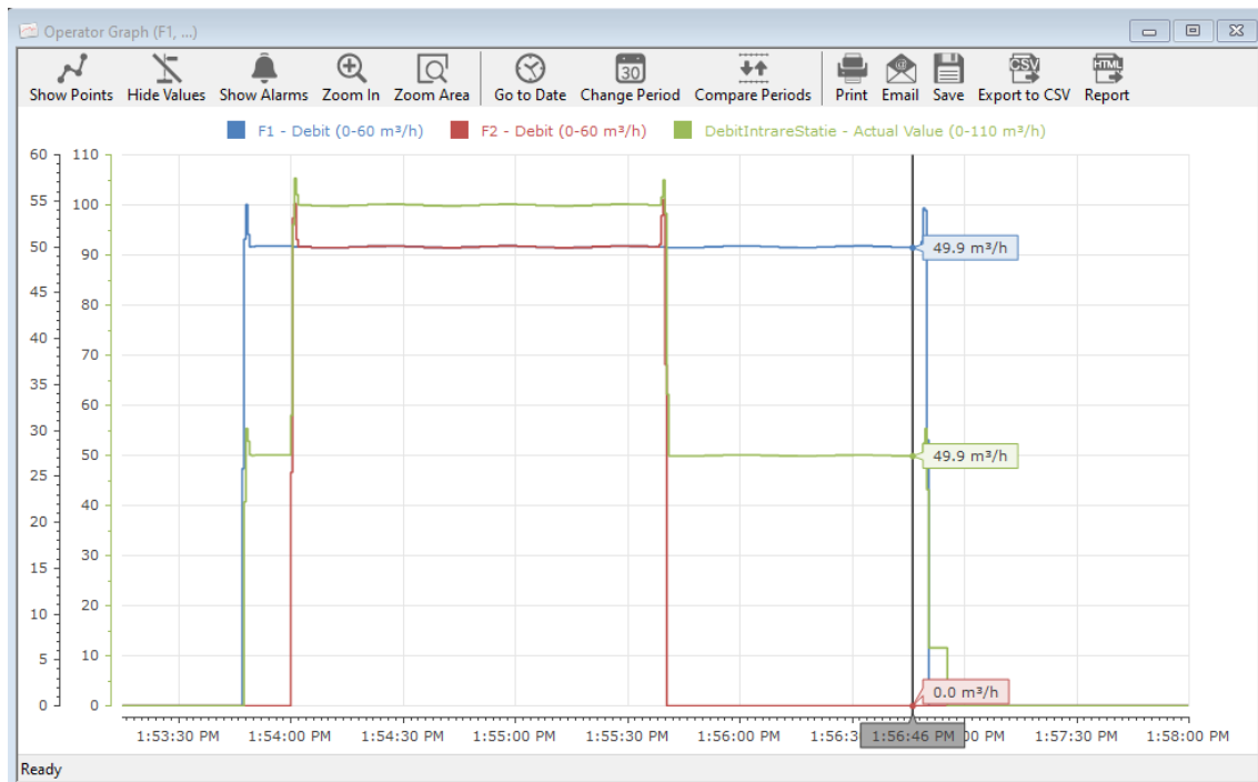
Figure 11. Time of SCADA operator intervention to stop borehole pump 1
